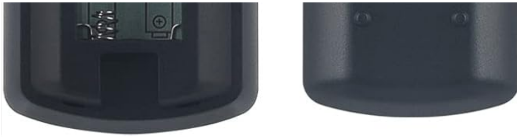
Figure 2: Battery compartment with cover removed, showing AAA battery slots.
