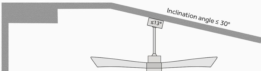
The ceiling fan can be tilted up to 13 degrees and can be installed on an inclined plane.
