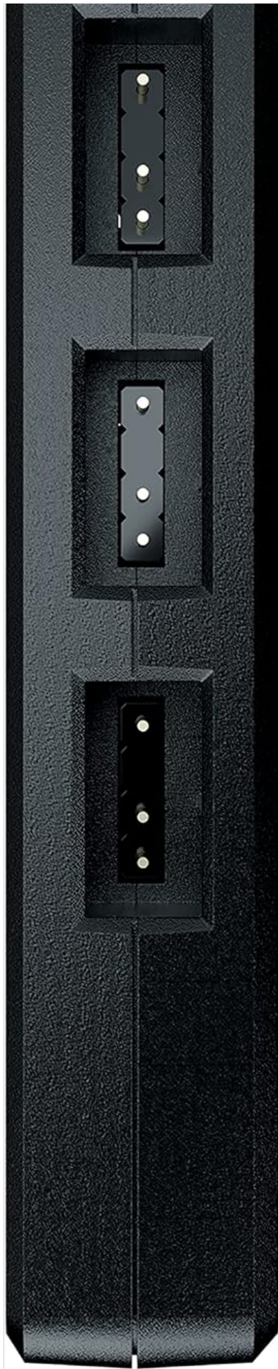
Figure 4: Opposite side view of the LED Controller A1, showing the three Addressable RGB (ARGB) headers for connecting LED devices.
