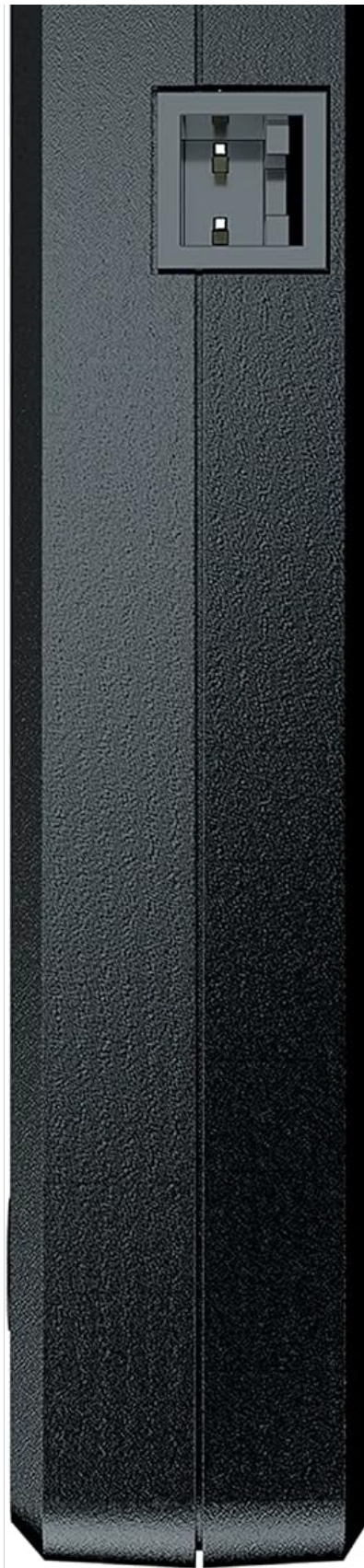
Figure 3: Side view of the LED Controller A1, highlighting the USB port for data connection to the PC and the power input port.
