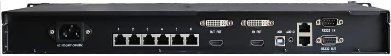
Figure 2.2: Rear panel of the MCTRL700, featuring the AC power input, six Gigabit Ethernet output ports (1-6), DVI IN/OUT, HDMI IN/OUT, USB control port, audio input, and RS232 IN/OUT ports for control and cascading.
