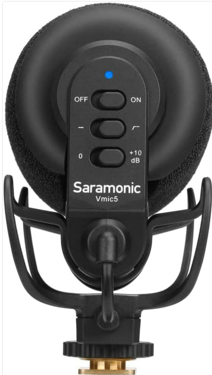
Image: A detailed view of the Saramonic Vmic5's control panel, highlighting the power button, 2-stage gain control (0dB, +10dB), and the 150Hz high-pass filter switch.
