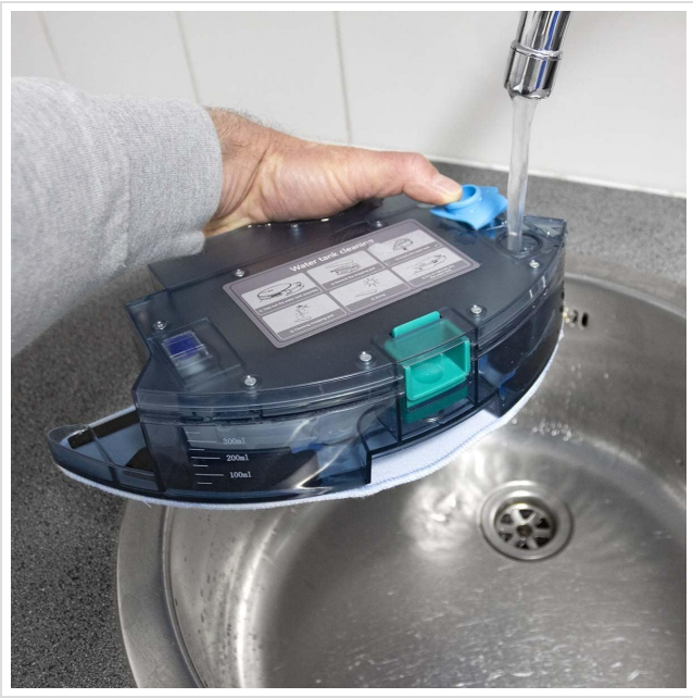
Image Description: A hand is shown holding the transparent water tank of the robot vacuum cleaner under a running water faucet, indicating the process of filling or rinsing the tank. The tank has measurement markings and a blue cap.
