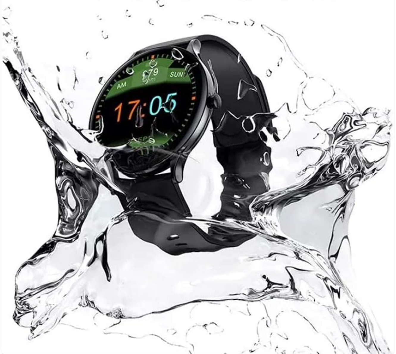
Figure 3.1: The QW13 Smartwatch demonstrating its IP67 waterproof design. While resistant to splashes and daily activities, it is not suitable for deep-sea diving, saunas, or hot baths.
