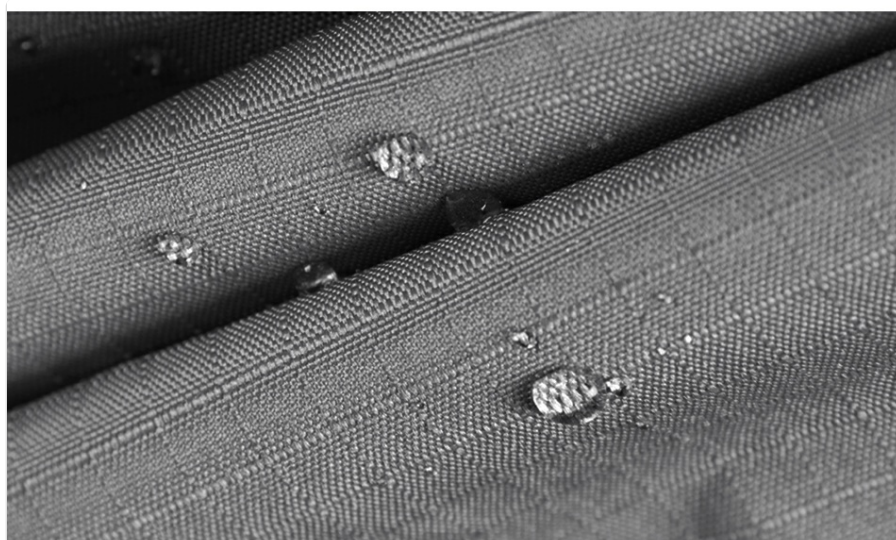
Image 6.1: Detail of the Rip-Lock fabric, highlighting its water-resistant properties.
