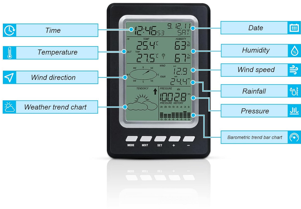
Figure 4: Detailed view of the LCD display, indicating the location of various data points and indicators.
