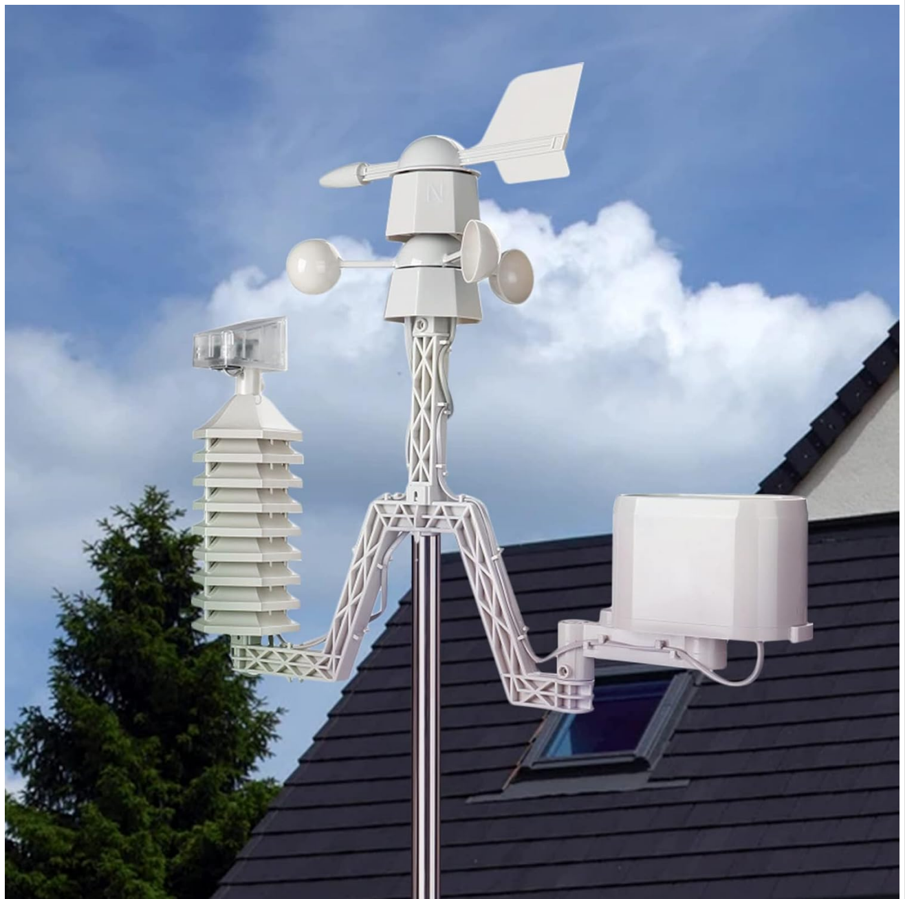
Figure 3: Example of the outdoor sensor unit installed on a rooftop, demonstrating an ideal elevated and unobstructed placement.
