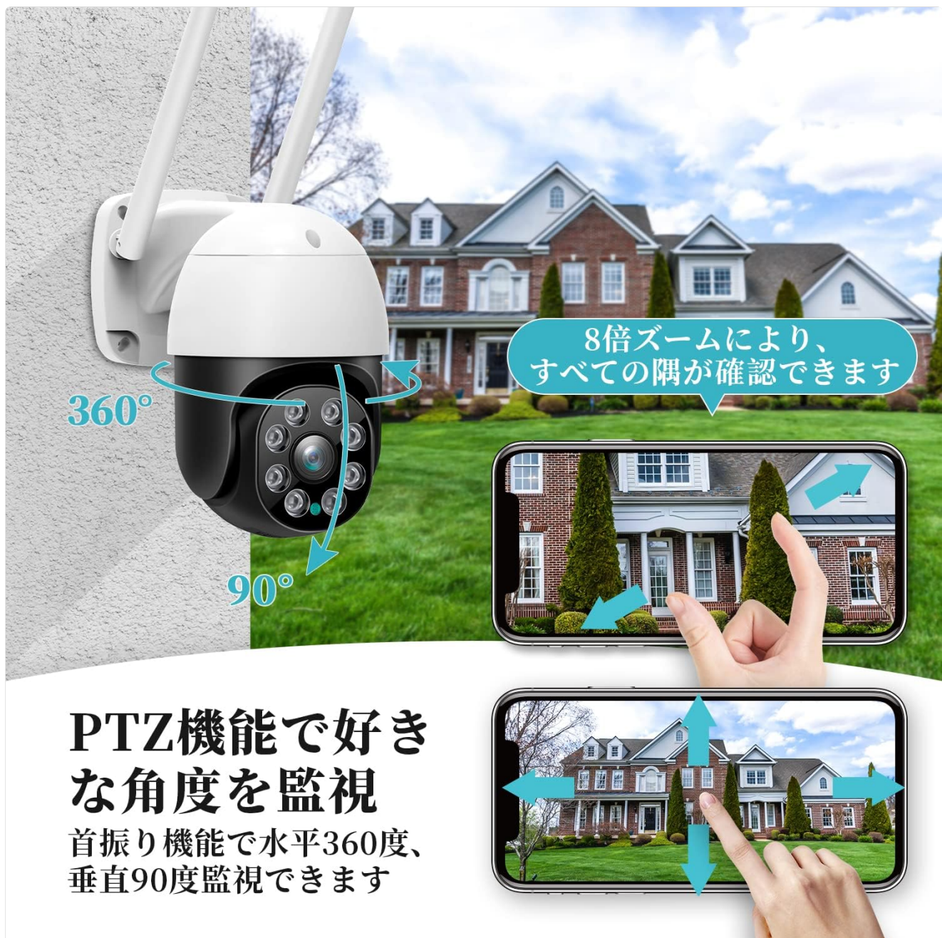
Figure 4.1: The camera offers 360° horizontal pan and 90° vertical tilt, controllable via the app to monitor any desired angle. It also features 8x digital zoom.
