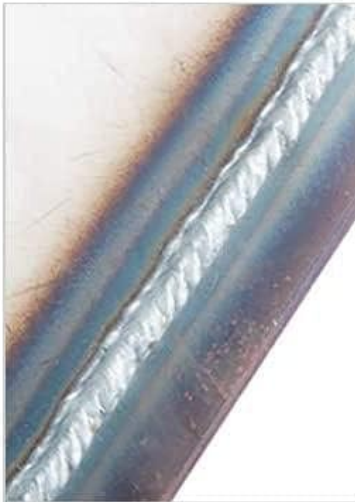
Welding of mixed gas 1mm cold rolled plate
