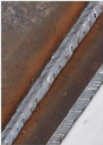
Gas welding of CO2 5mm carbon steel plate
