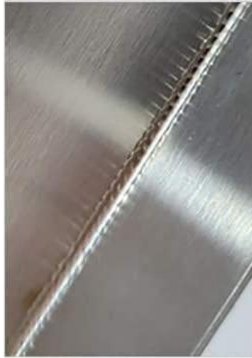
Precision cold welding 0.8mm stainless steel plate
