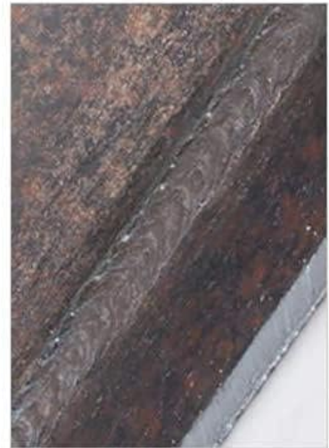
Flux welding 5mm carbon steel plate
