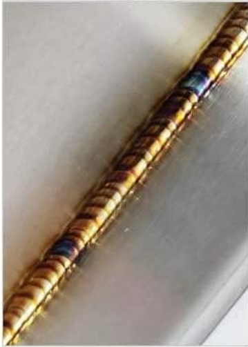
TIG hot welding 3mm stainless steel plate
