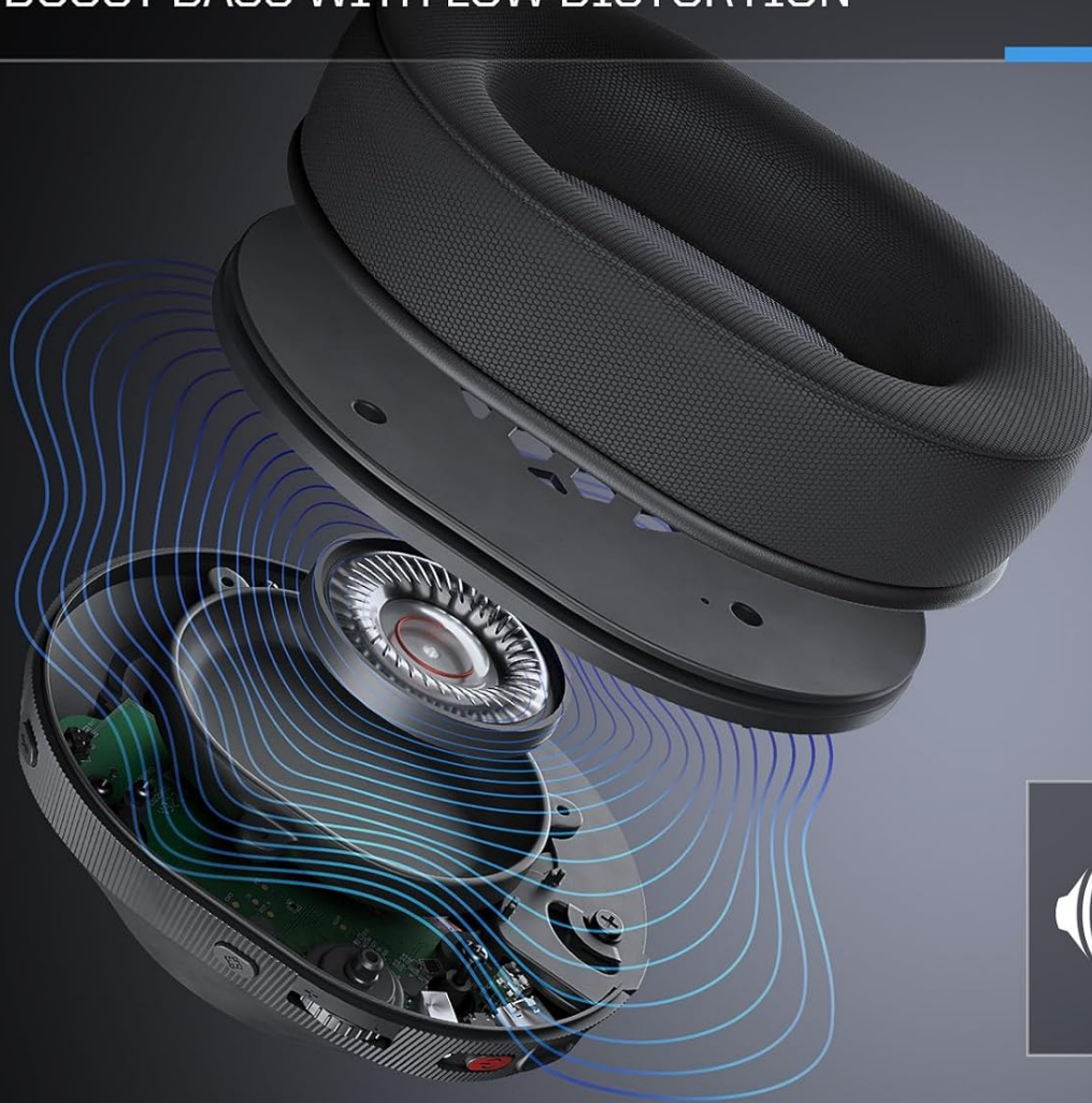
Figure 4: The 40mm drivers deliver high-quality game audio.
