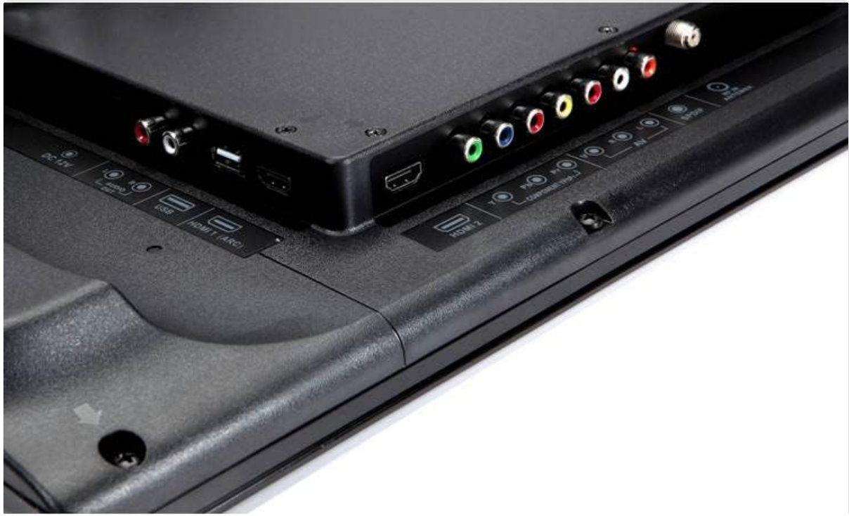
Figure 3: Rear Panel Connections. This close-up image displays the rear input and output ports of the Jensen JTV3220DC. Visible connections include HDMI (with ARC support), USB, Composite Video, Component Video, RF, and various audio inputs and outputs, indicating comprehensive connectivity options.
