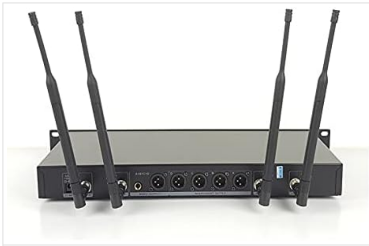
Figure 4.2: Rear view of the receiver unit, highlighting the four individual XLR outputs (CHANNEL A, B, C, D), the 1/4" mixed output, and the antenna input ports.
