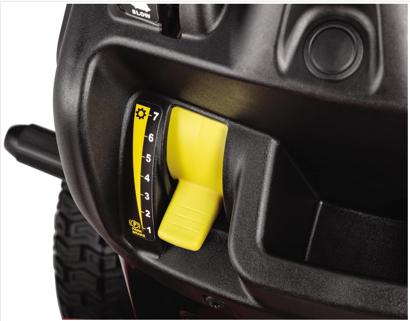
Image: Detailed view of the yellow 7-speed manual transmission selector lever, indicating different speed settings and a park brake position.
