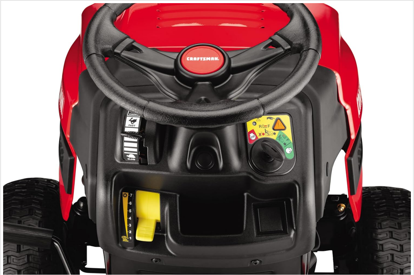
Image: Close-up view of the operator's console, showing the steering wheel, ignition switch, and controls for engine speed and choke.
