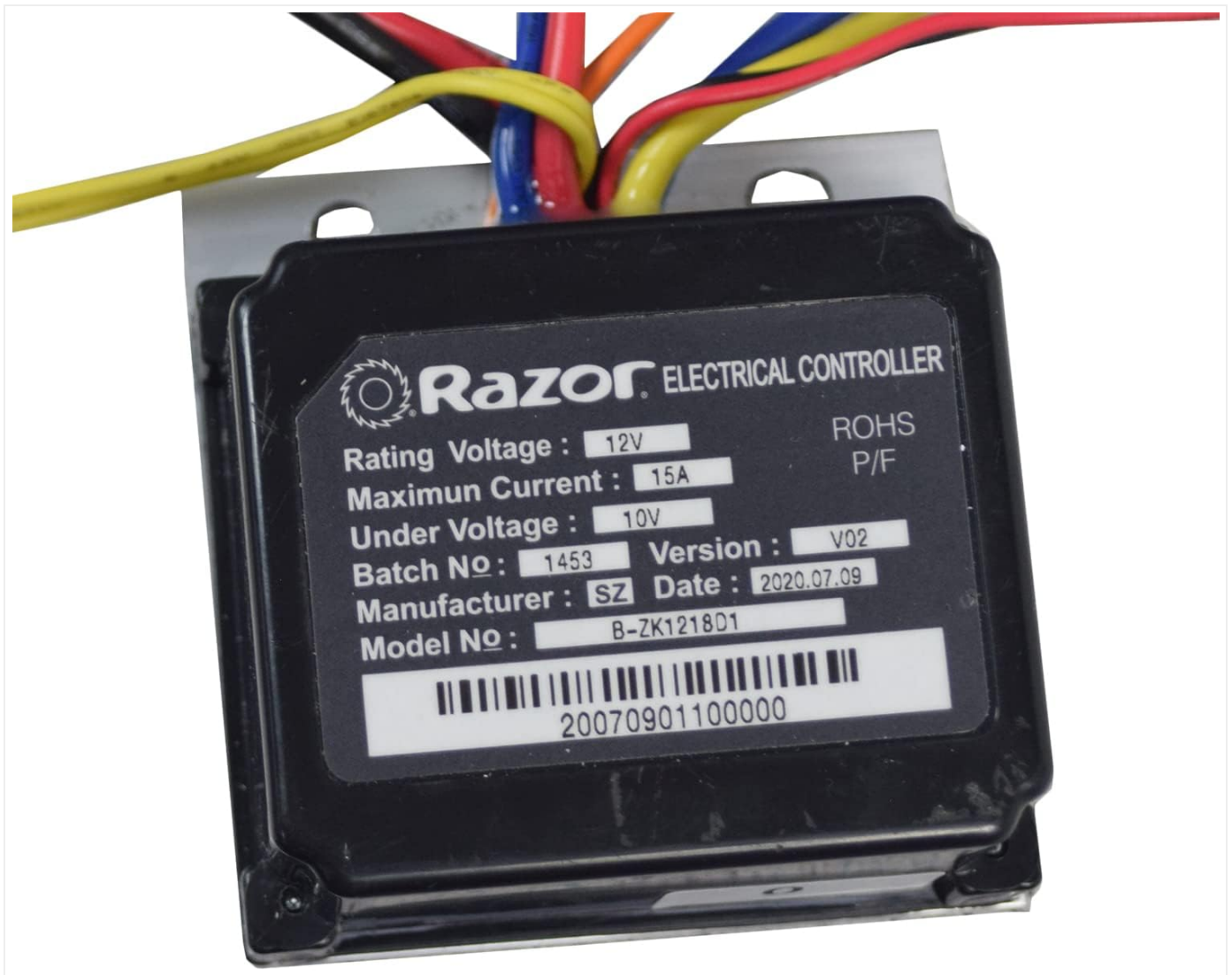
Figure 2: Close-up view of the control module's label. The label clearly shows 'Razor Electrical Controller', 'Rating Voltage: 12V', 'Maximum Current: 15A', 'Under Voltage: 10V', 'Model No: B-ZK1218D1', and a barcode with the number 20070901100000, confirming the module's specifications and identification.
