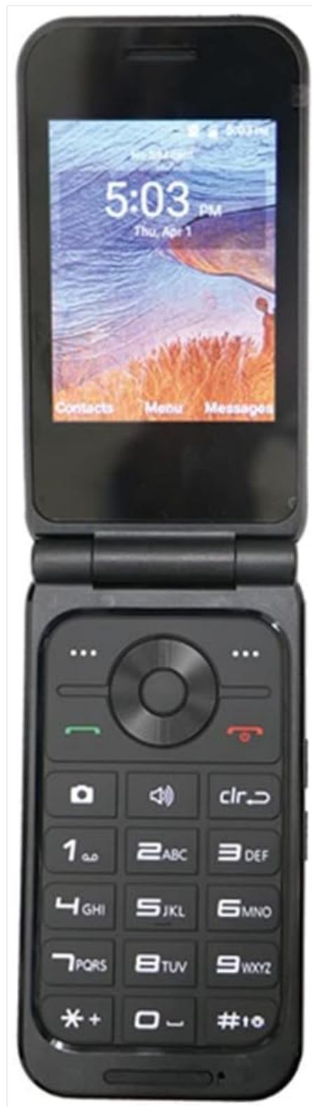
Figure 4.2: Front view of the ZTE Cymbal U Link II Z2335CC when open, revealing the main screen and the alphanumeric keypad.
