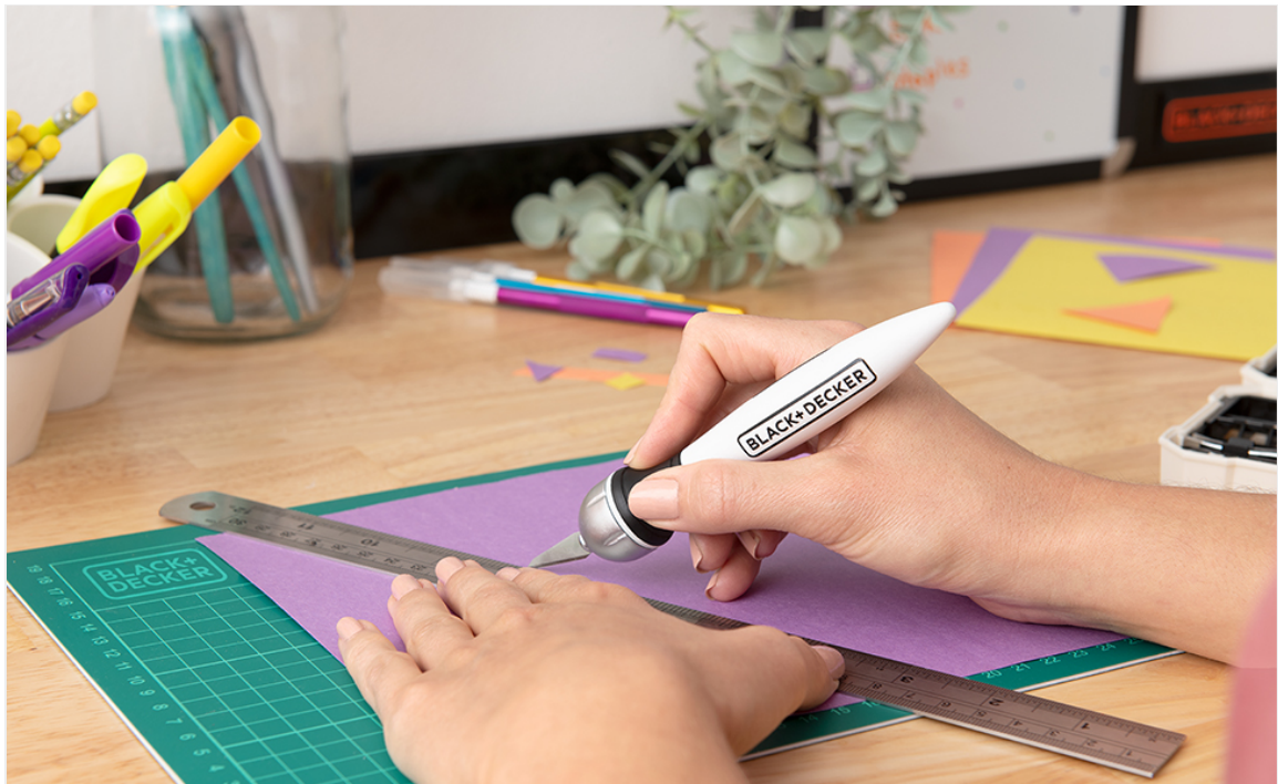
Image 5.1: Demonstrating the use of the hobby knife with the metal ruler and cutting mat for precise cuts.
