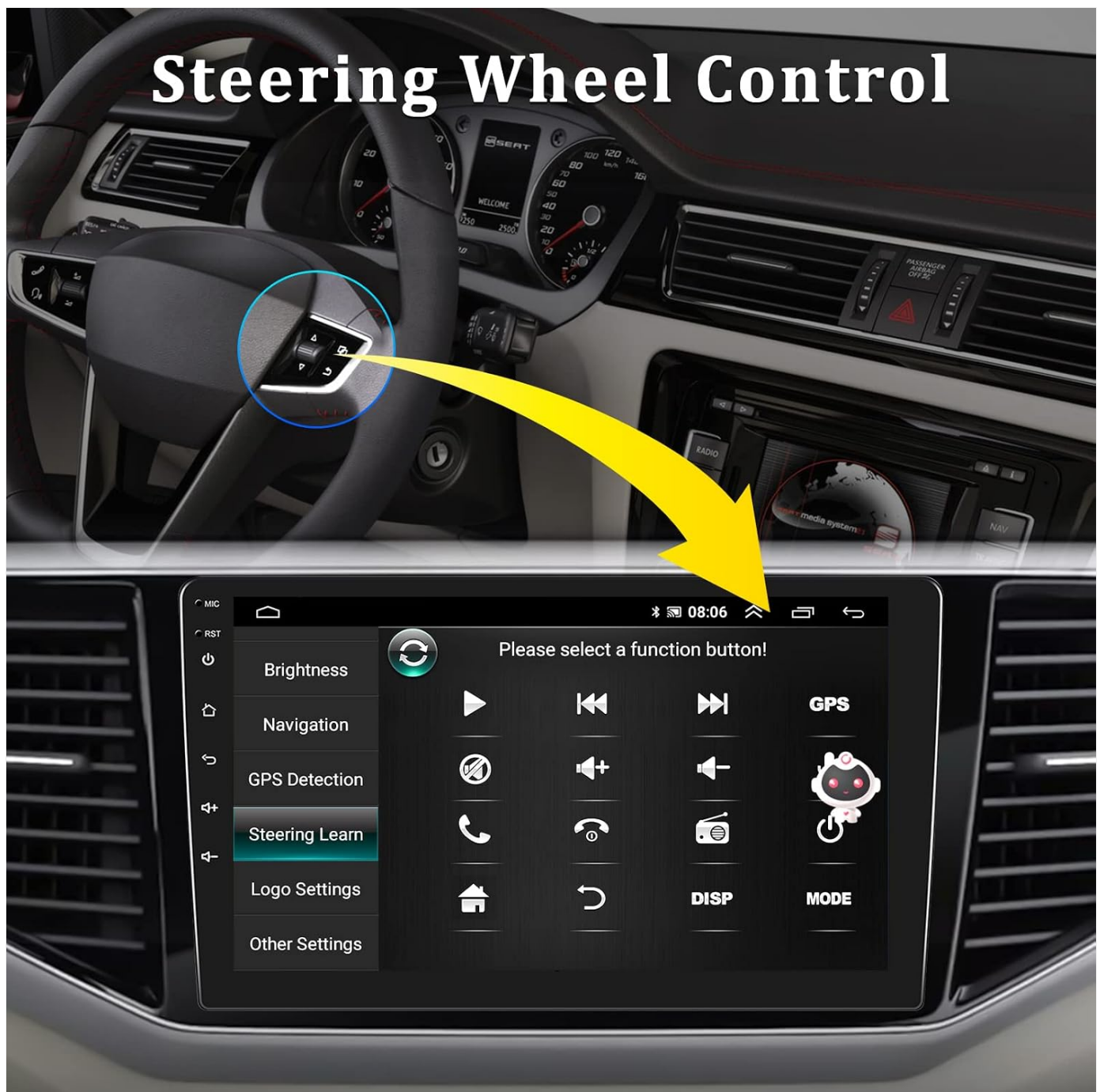
Figure 6.4: Image demonstrating the steering wheel control setup interface, showing how to assign functions to physical buttons on the steering wheel.
