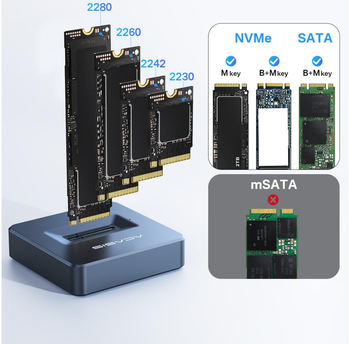
Image: Visual representation of supported M.2 NVMe and SATA SSD form factors and key types.
