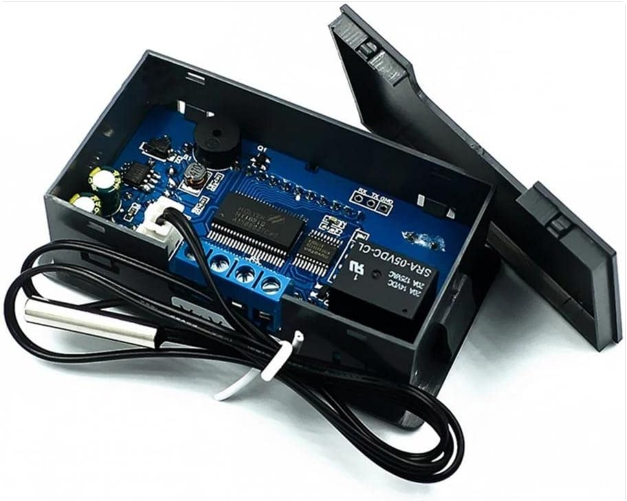
Figure 3.3: Internal view of the XY-WT01, showing the circuit board, relay, and terminal blocks for power and load connections.
