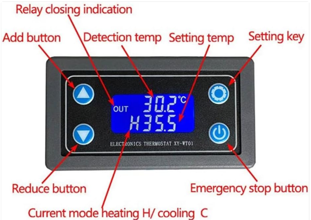
Figure 3.4: Labeled diagram of the XY-WT01's front panel, indicating the functions of each button and display element: Relay
