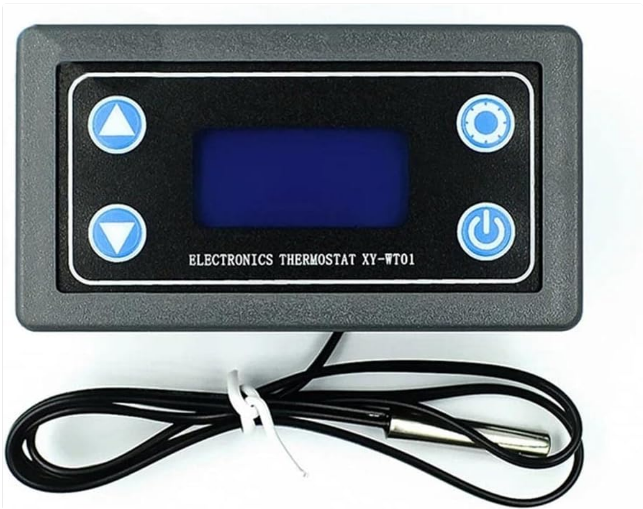
Figure 3.2: Close-up front view of the XY-WT01, highlighting the LED display and the four control buttons: Up, Down, Set, and Power/Emergency Stop.
