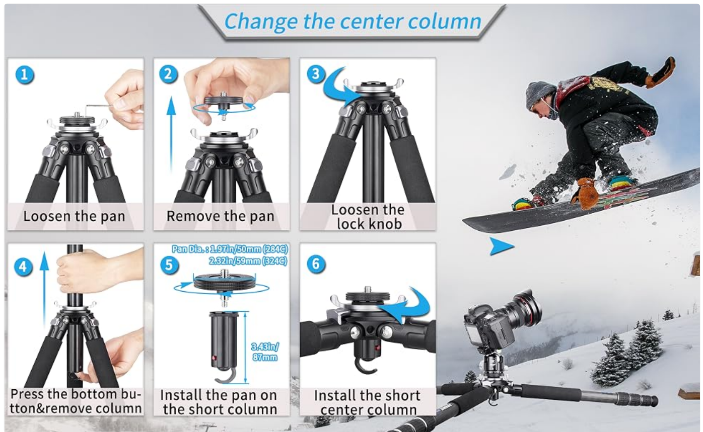
Image: Step-by-step guide on how to remove the standard center column and install the shorter center column for low-angle shooting.
