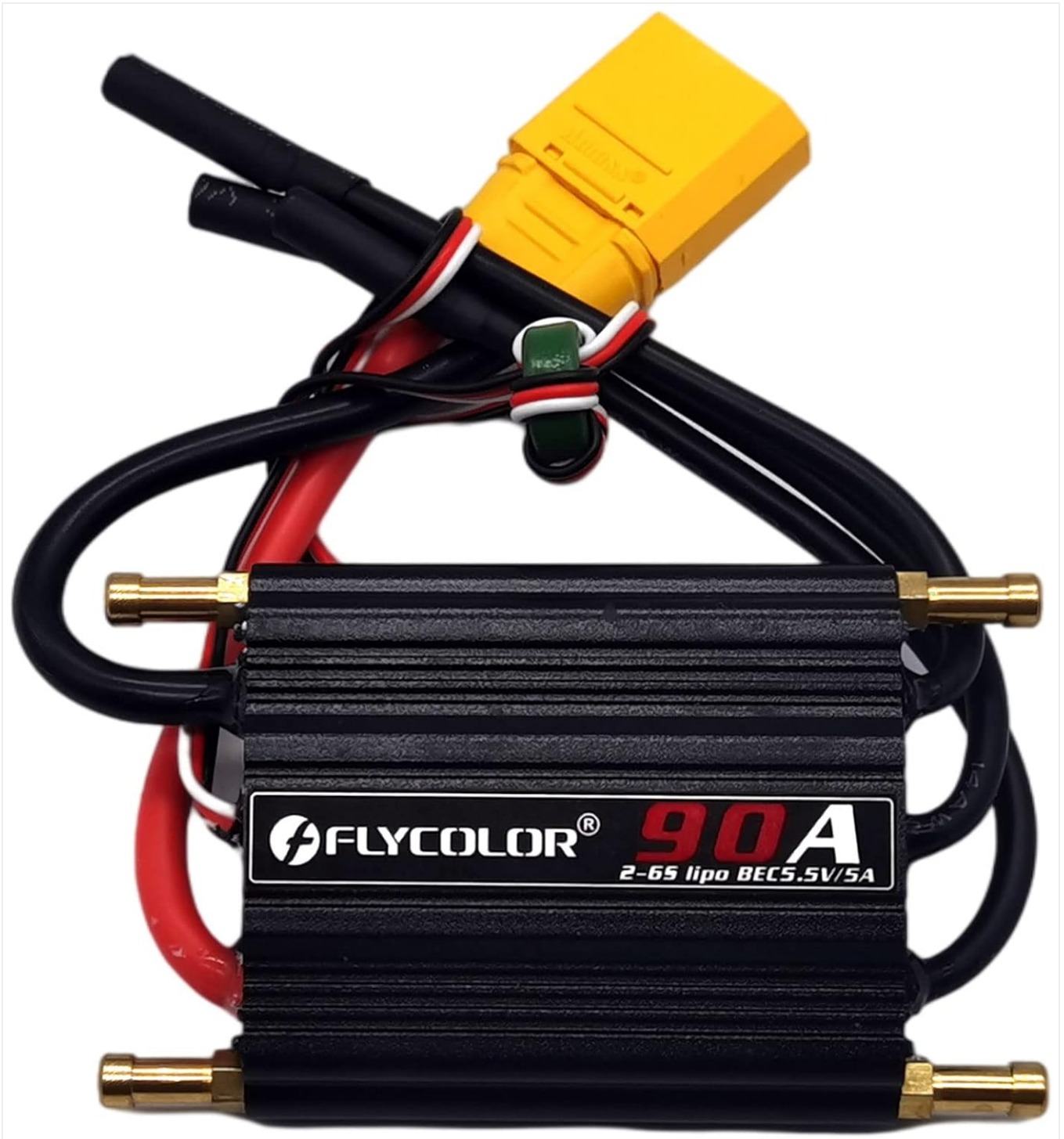
Figure 4.1: Front view of the FLYCOLOR 90A Waterproof Brushless ESC, showing the main unit with attached power and motor wires, and an XT90 battery connector.
