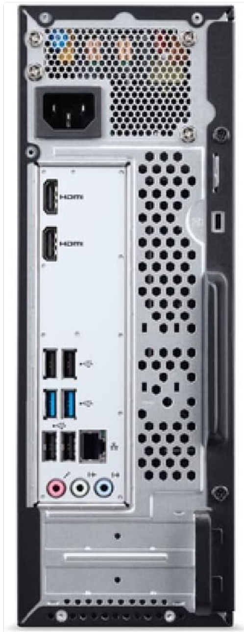
Figure 3.1: Rear view of the Acer Aspire XC Desktop PC, highlighting the power input, HDMI ports, USB ports, Ethernet port, and audio jacks.
