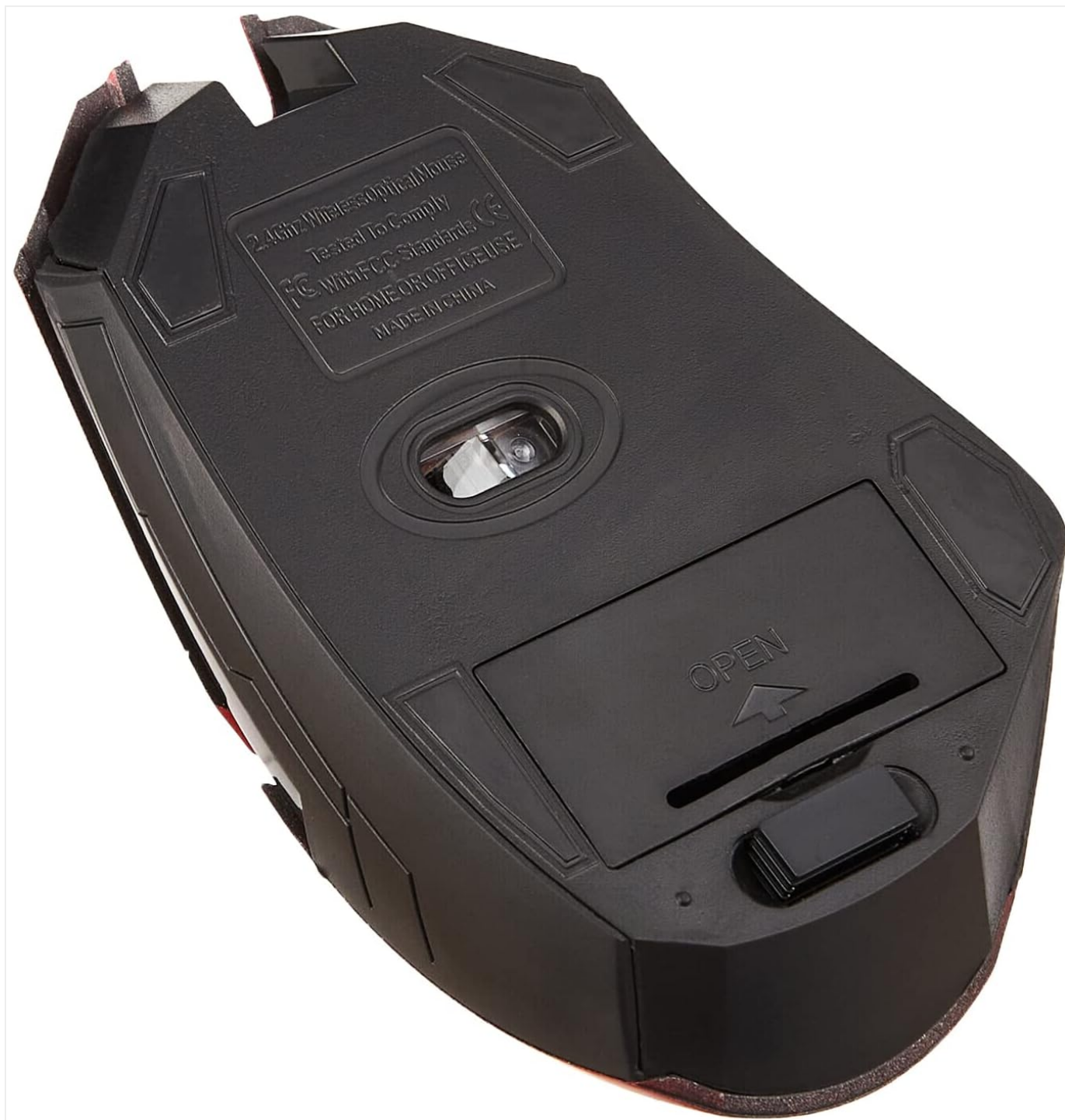
Figure 3.2: Bottom view of the iMICE E-1700 Wireless Mouse. This image highlights the optical sensor, the battery compartment with an "OPEN" indicator, and the power ON/OFF switch. The bottom surface is black with regulatory markings.
