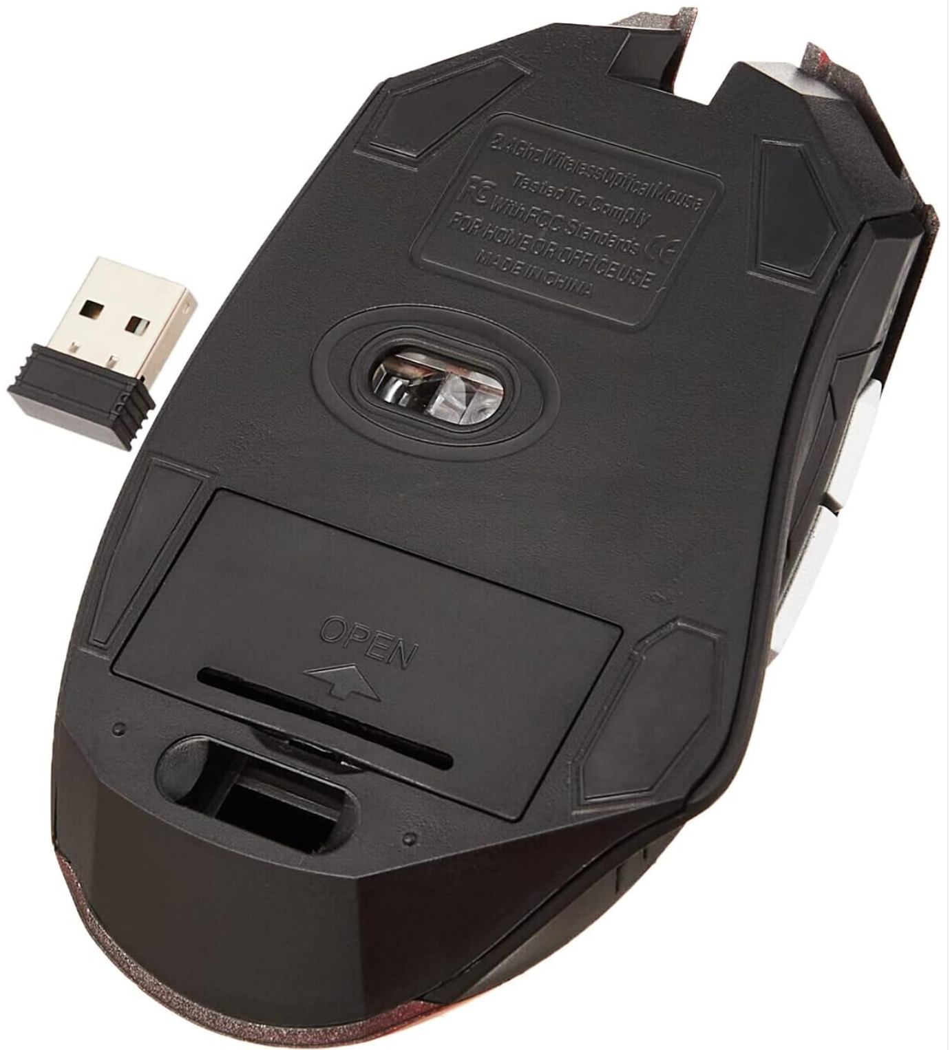
Figure 3.3: Bottom view of the iMICE E-1700 Wireless Mouse with the USB receiver. This image shows the USB receiver detached from its dedicated storage slot next to the battery compartment, ready for connection to a computer.
