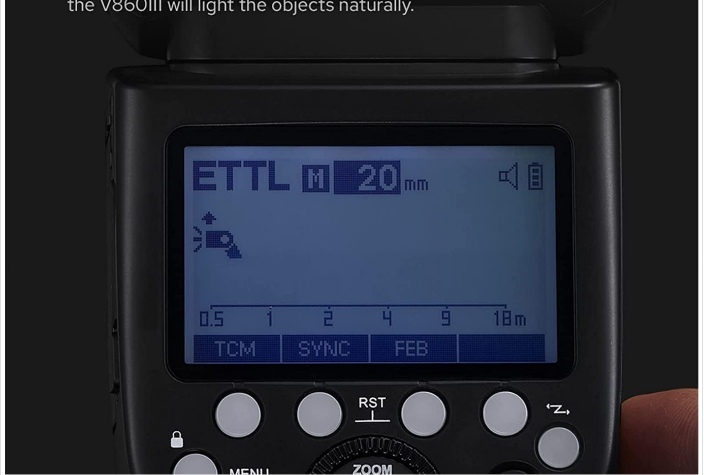
Figure 6: The flash head can be zoomed from 20mm to 200mm, either automatically or manually, to optimize light coverage for various focal lengths.
