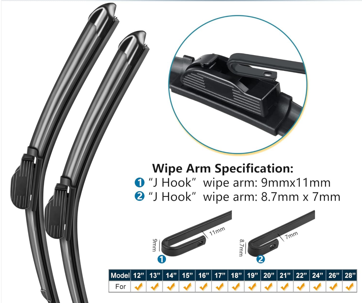
Image 2.2: Wiper arm specification for "J Hook" type.
