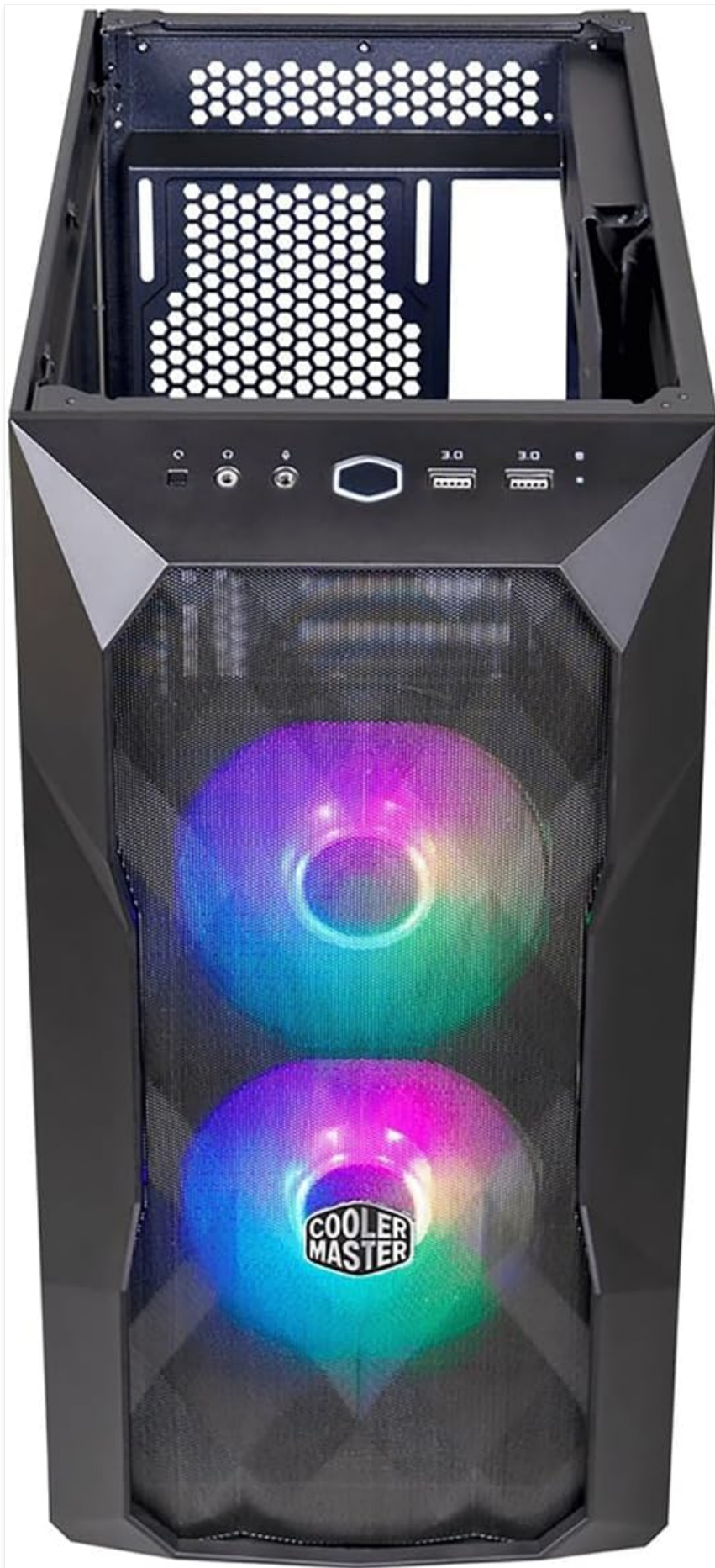
Figure 4.1: Top I/O panel with power button, USB ports, and audio jacks.
