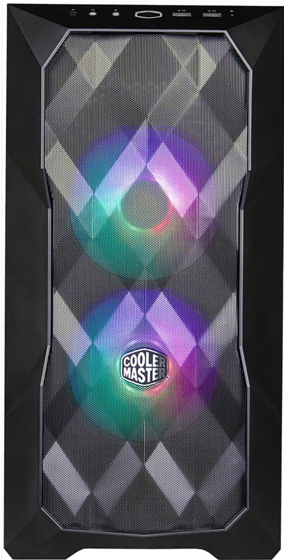
Figure 2.1: Front view showcasing the polygonal mesh and ARGB fans.
