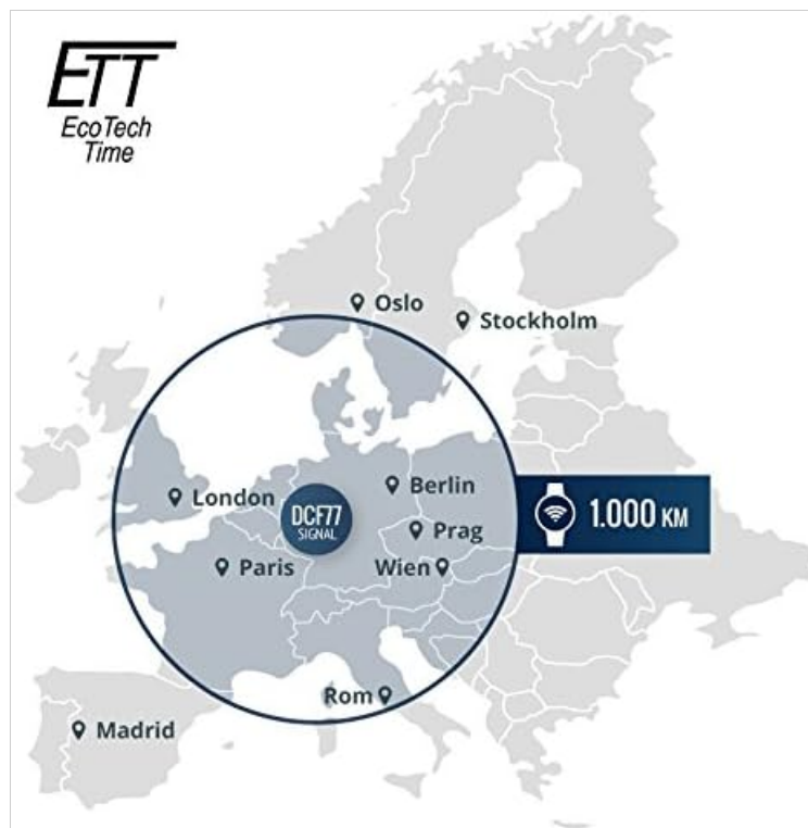
Image 4: DCF 77 Signal Reception Map. This map illustrates the approximate 1000 km reception range of the DCF 77 radio signal, originating from Mainflingen, Germany. Major European cities within this range, such as London, Paris, Berlin, and Rome, are indicated, demonstrating the watch's ability to automatically synchronize time across a wide area.
