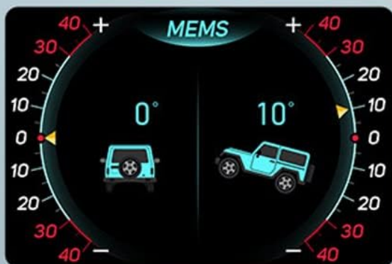
Figure 5: The G-Sensor Slope Meter display, showing real-time left/right tilt, uphill, and downhill angles, beneficial for off-road driving.
