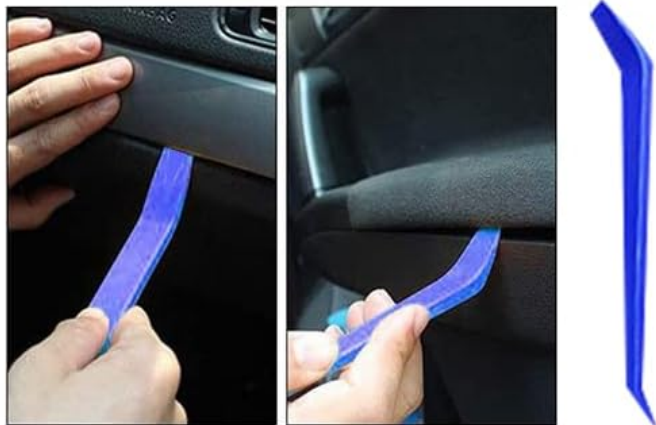
Crowbar Hiding the OBD cable in the A-pillar
