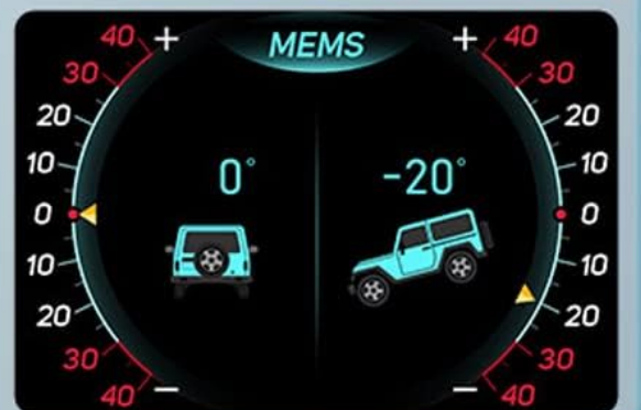
Figure 5: The G-Sensor Slope Meter display, showing real-time left/right tilt, uphill, and downhill angles, beneficial for off-road driving.
