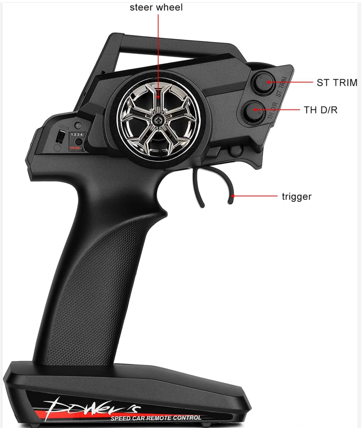
Image 4.1: Remote control layout, showing the steer wheel, trim adjustments, and trigger.
