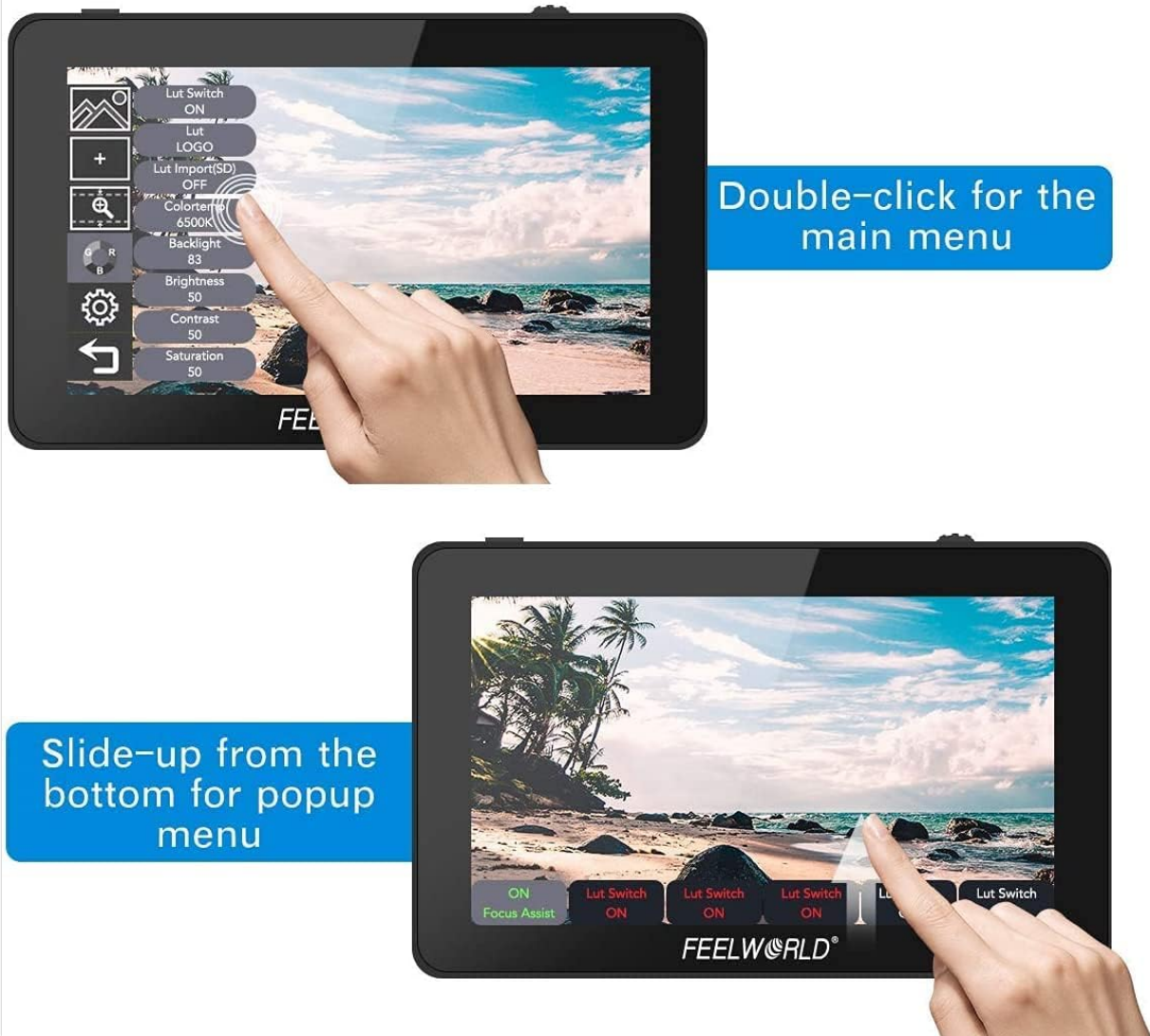
Figure 4.1: Illustration of touch screen controls on the FEELWORLD F6 PLUS. The top image shows a double-click action to access the main menu, while the bottom image demonstrates a slide-up gesture from the bottom for a popup menu.
