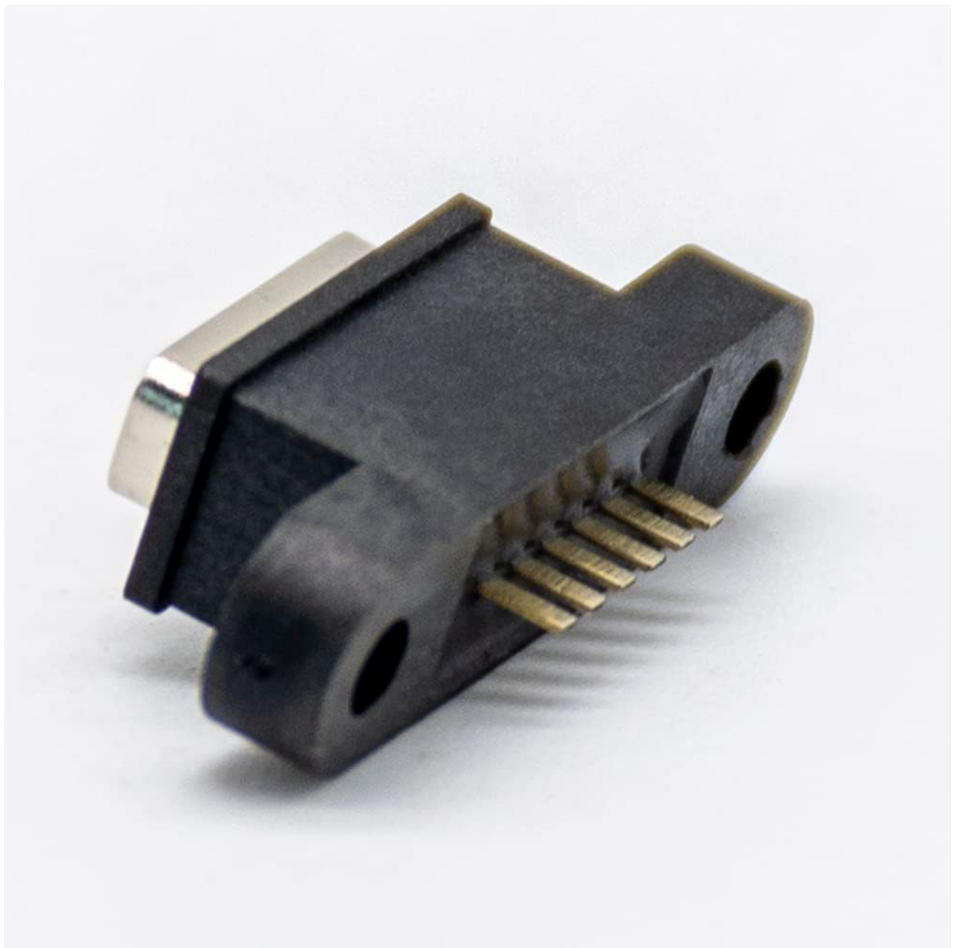
Figure 1.2: Angled view showing the 6 SMT pins for PCB integration.
