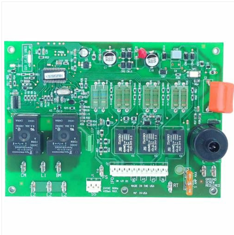
Figure 1: The ClimaTek ICM291 Furnace Control Circuit Board. This image displays the green circuit board with various electronic components, including relays, capacitors, resistors, and connectors. The board is rectangular with mounting holes in each corner.
