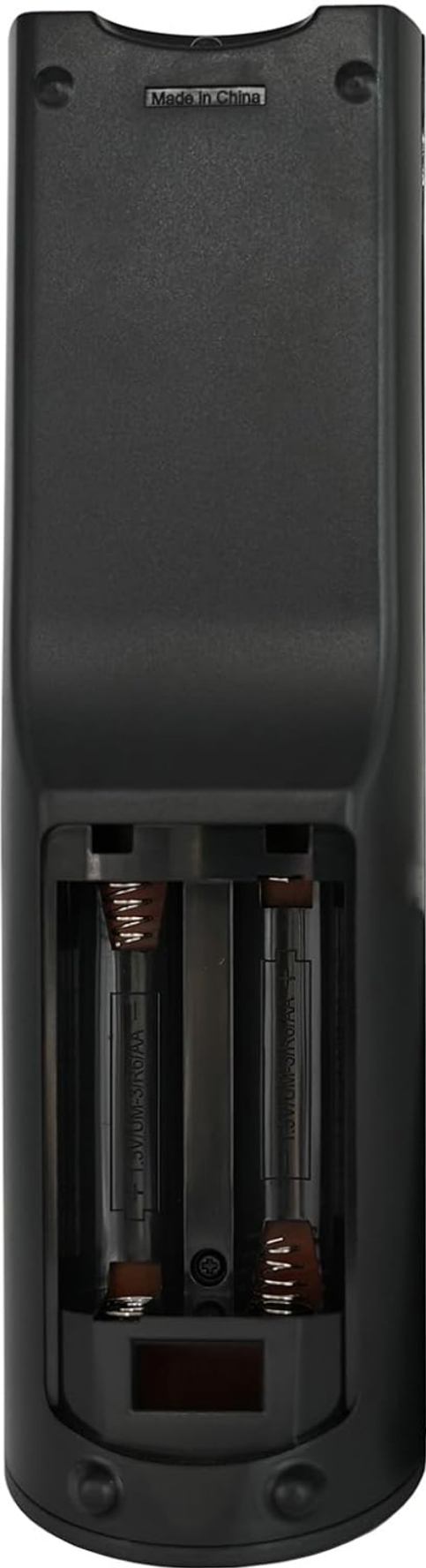
Figure 2.1: Battery compartment requiring two AA batteries.
