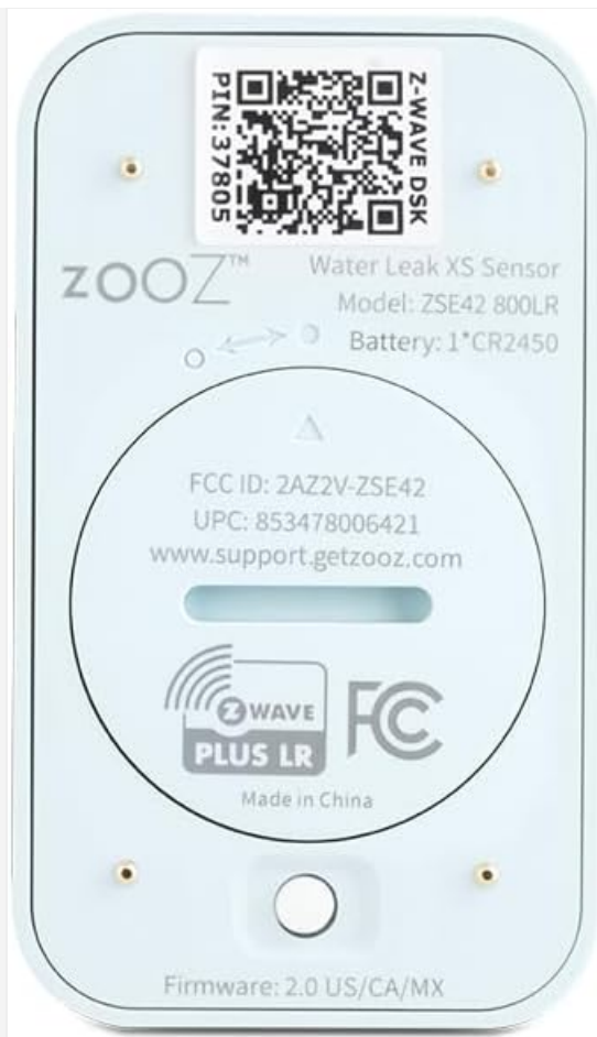
Image: The back of the Zooz Water Leak XS Sensor, displaying a QR code for SmartStart, the model number ZSE42 800LR, battery type, FCC ID, UPC, and Z-Wave Plus LR certification logos.
