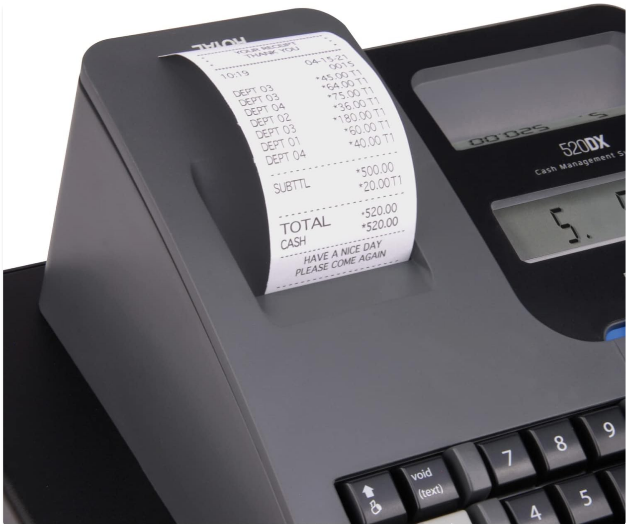
Figure 3: Detailed view of the thermal printer and receipt paper output.
