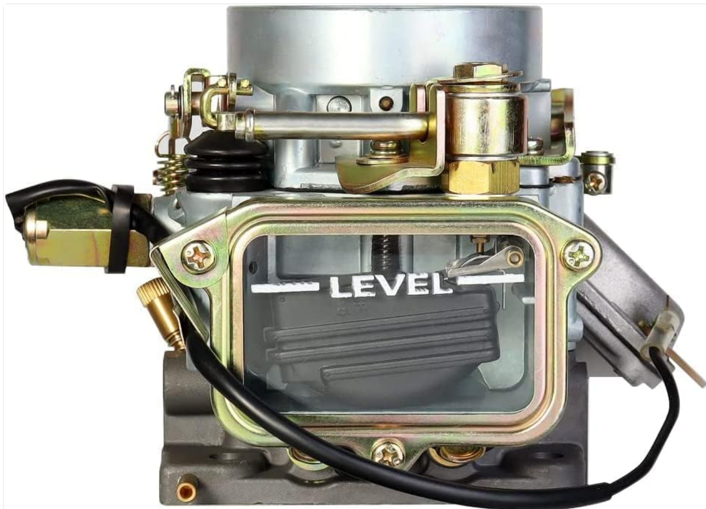
Figure 2.2: Front view of the carburetor, showing the transparent fuel level window for easy inspection.
