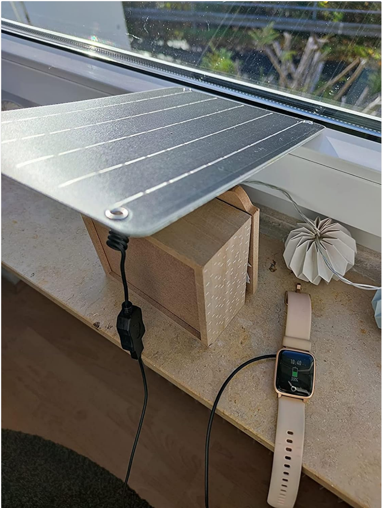
Figure 5: Smartwatch charging using the solar panel.
