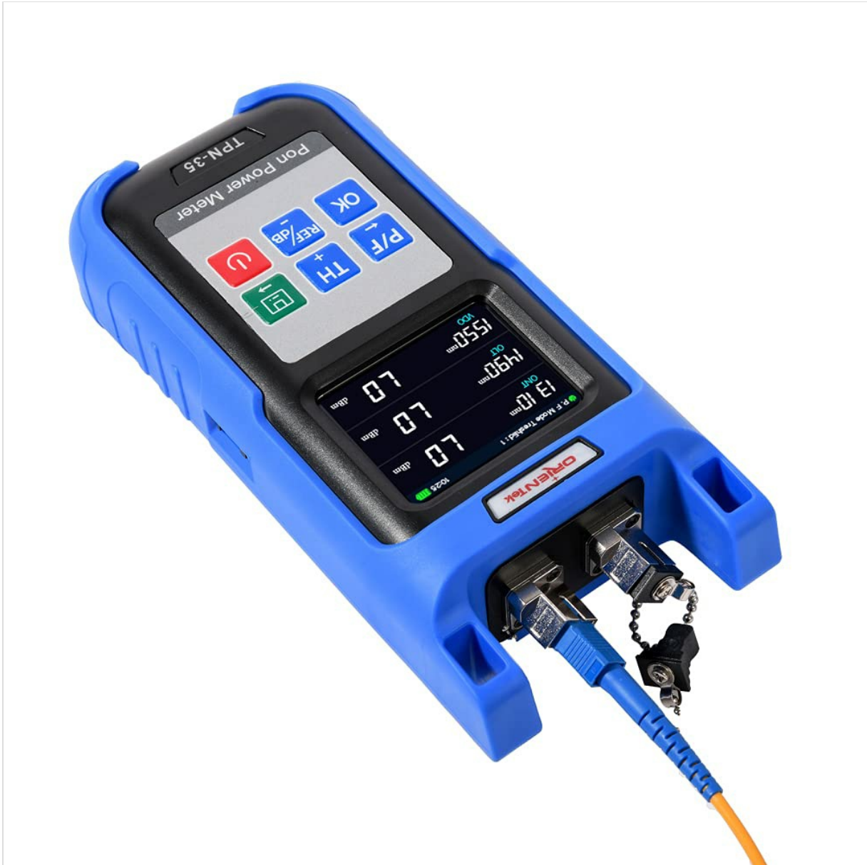
Figure 5: The TPN-35 device shown with a blue fiber optic cable connected to one of its APC input ports, ready for testing.
