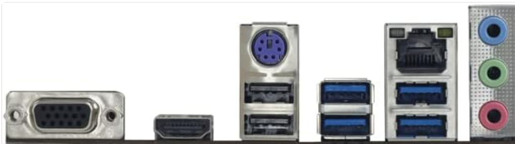
Figure 3.3: Rear Input/Output (I/O) panel of the motherboard, including video outputs, USB ports, and network port.
