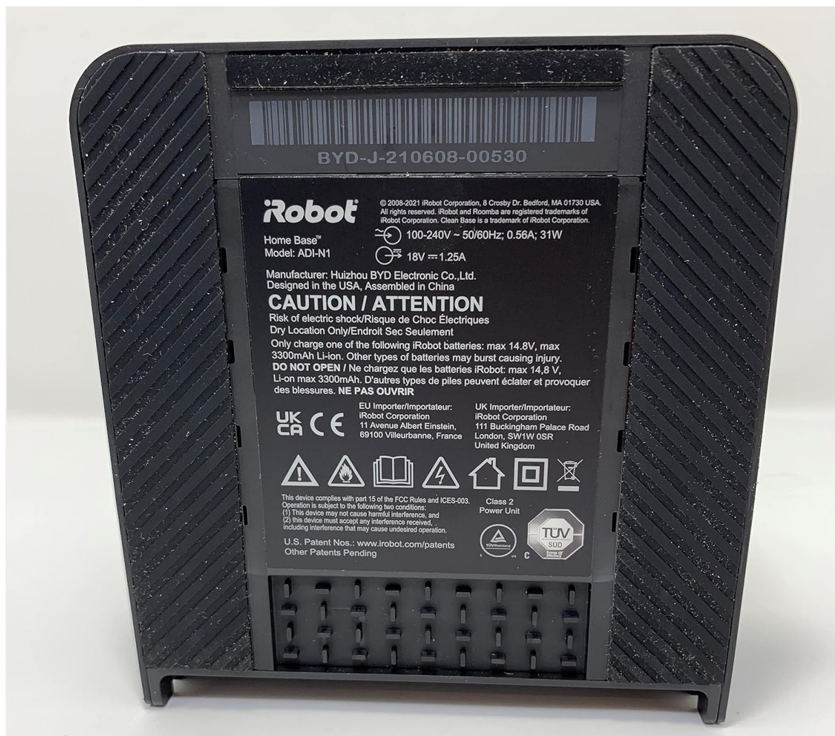
Figure 8.1: The bottom label of the charging dock, displaying model number ADI-N1 and electrical specifications (18V, 1.25A).
