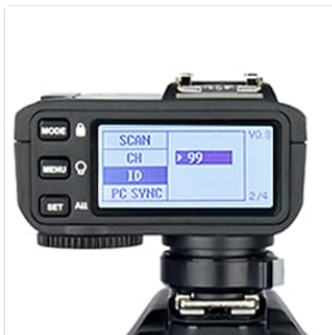
Figure 4.2.2: Screen displaying channel and wireless ID settings.
