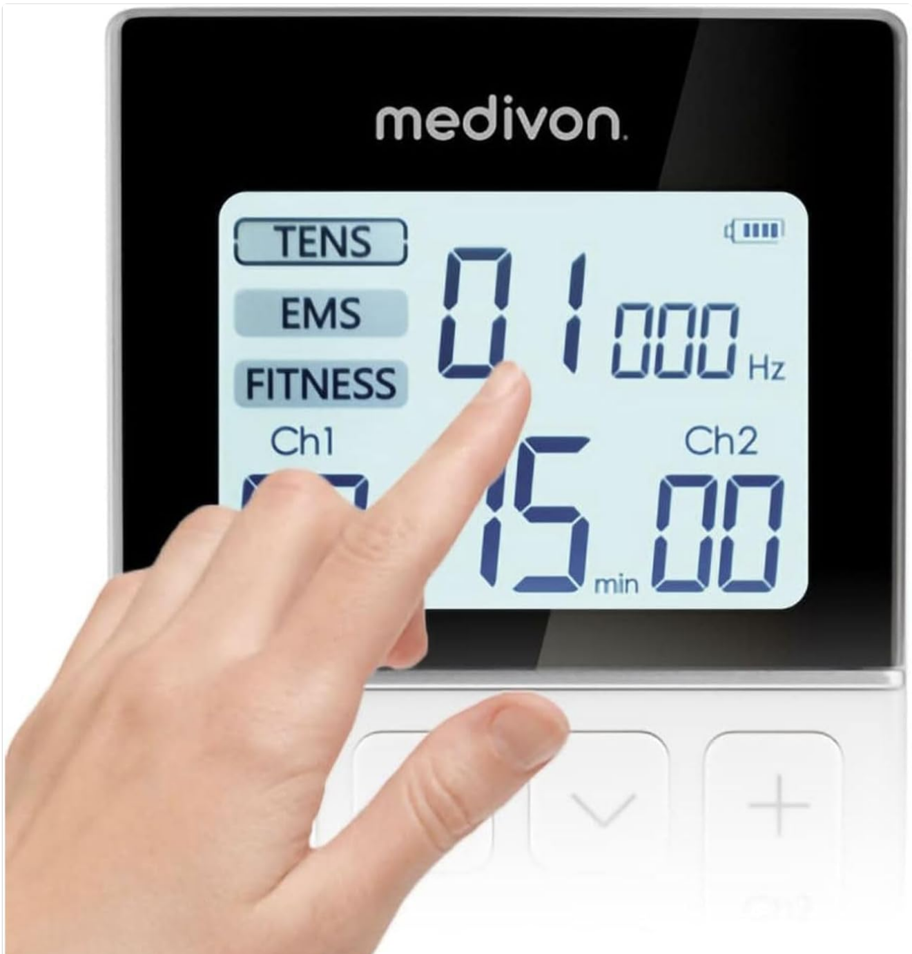
Figure 2: Close-up of the Medivon Stream PRO LCD display, showing program selection (TENS, EMS, FITNESS), frequency, and time settings. A finger is shown interacting with the screen.
