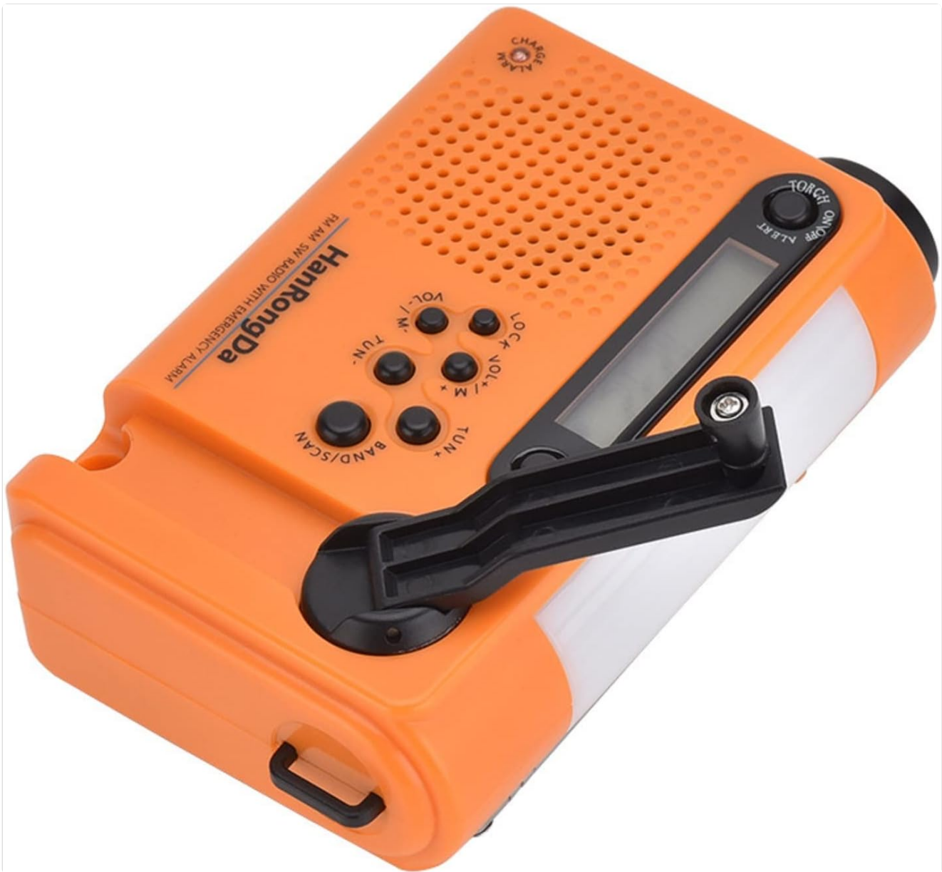
Figure 4.2: Hand-crank for emergency power generation.
