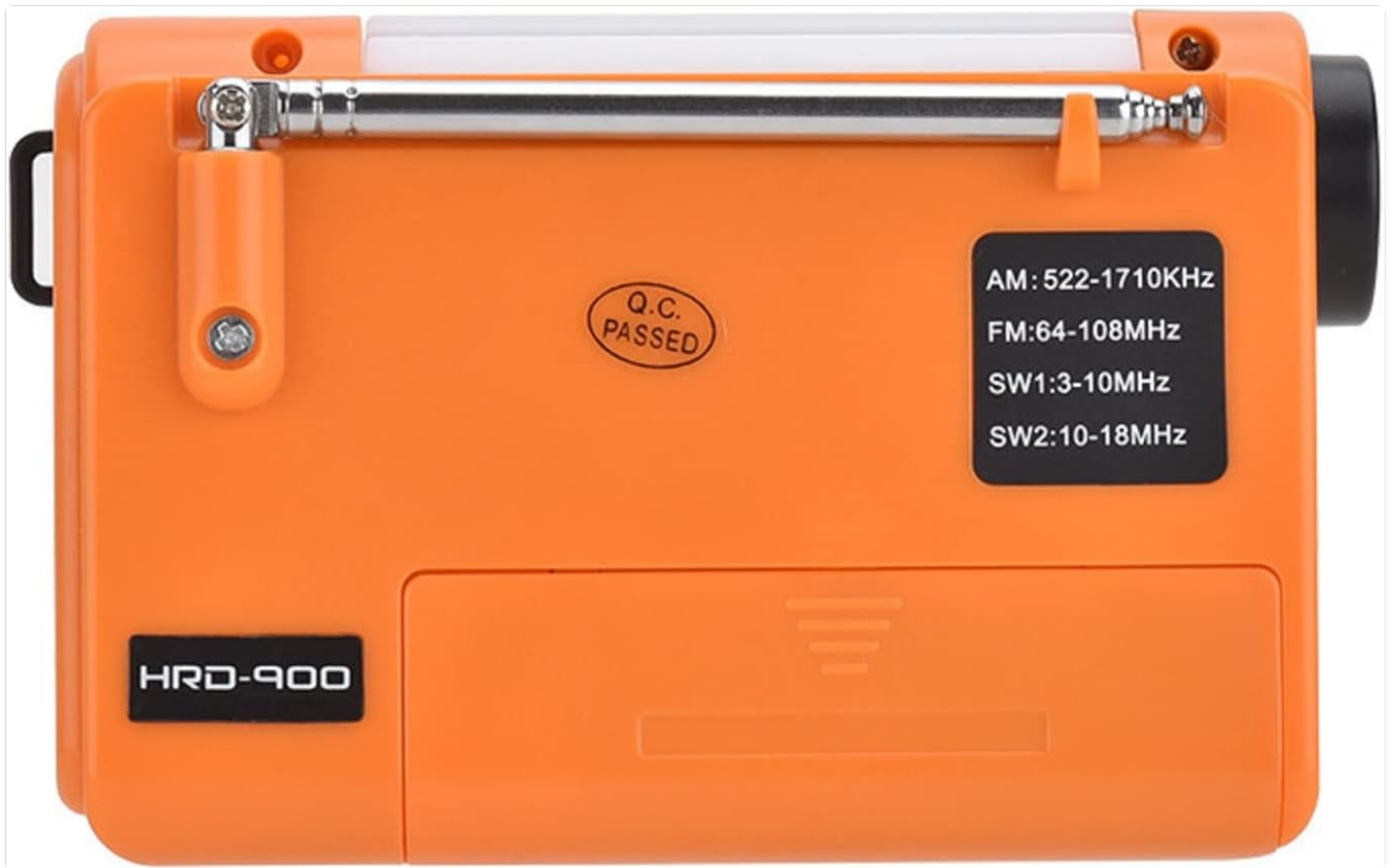
Figure 8.2: Back view showing frequency ranges and model number.
