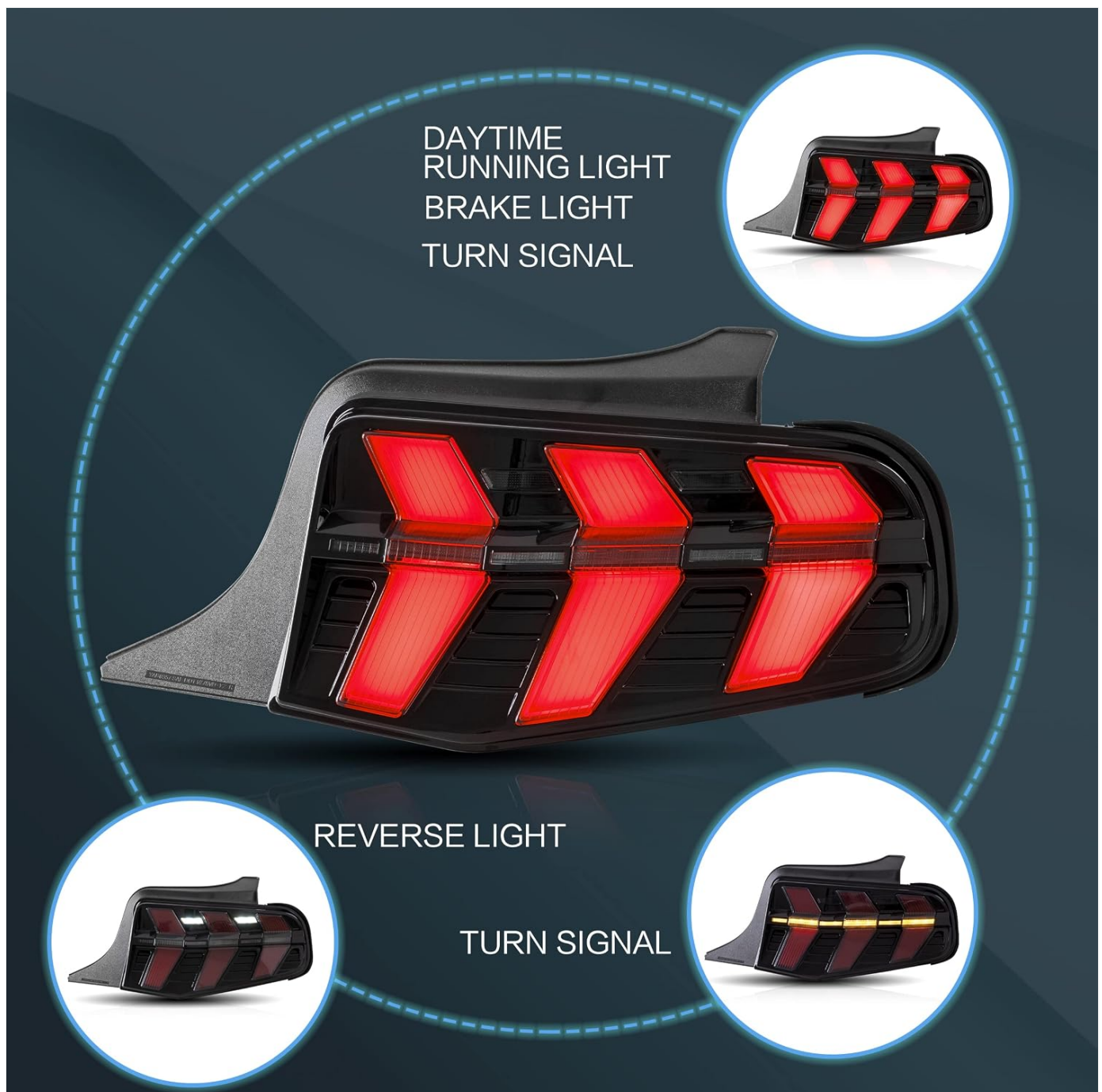
Image 2.1: Illustration of taillight functions including running, brake, turn, and reverse lights.
