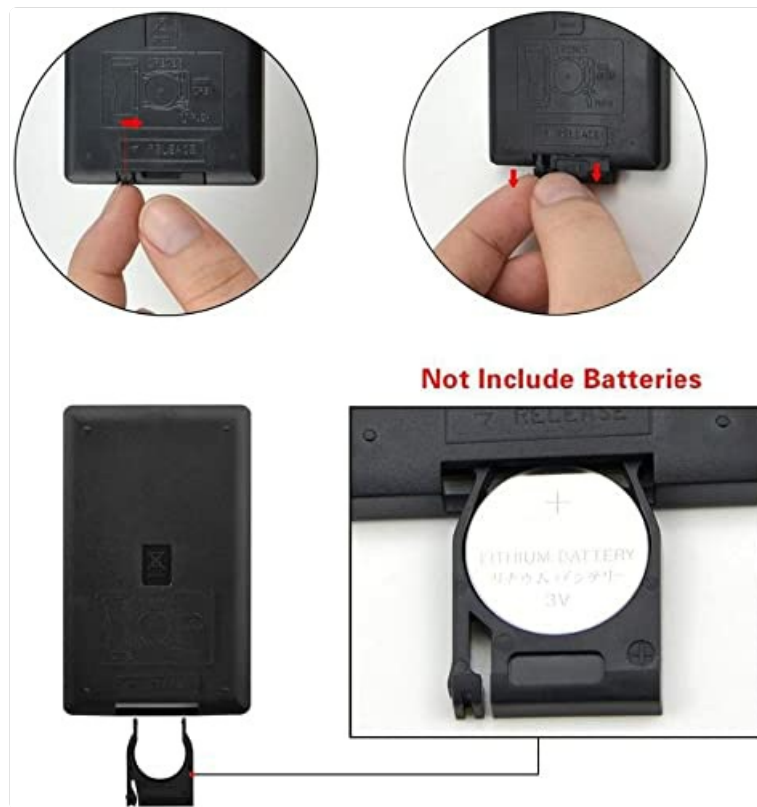
Image 2.2: Steps for installing the 3V lithium battery into the remote control.
