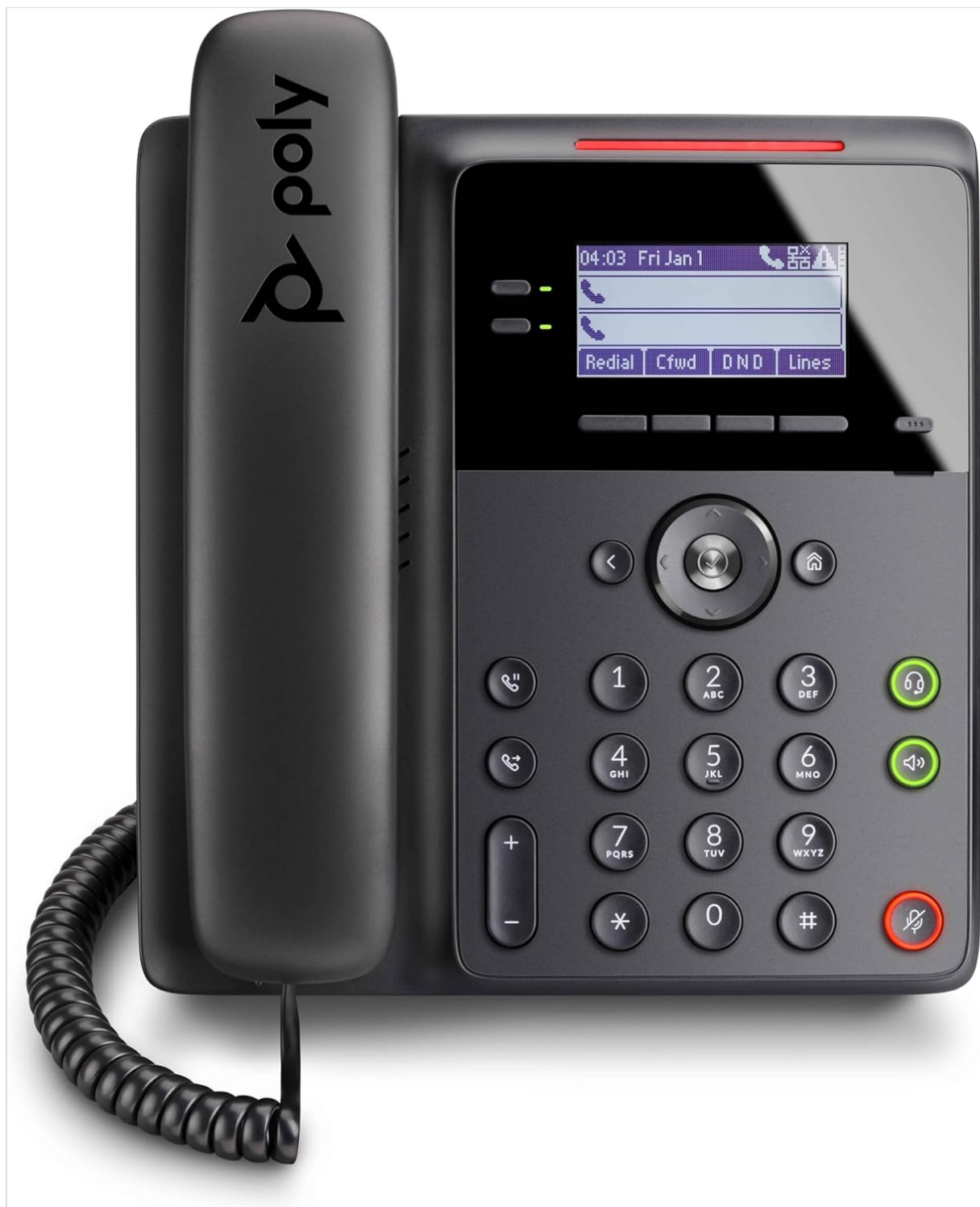
Image 4.0.1: Front view of the Poly Edge B20 IP Desk Phone with illuminated keys.
