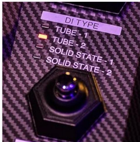
Image: Close-up of the DI Type selection area on the Zoom B6, showing indicators for Tube-1, Tube-2, Solid State-1, and Solid State-2.
