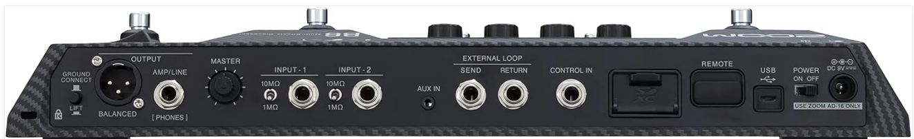
Image: Rear panel of the Zoom B6, showing various input and output jacks for connecting instruments, amplifiers, PA systems, and computers.
