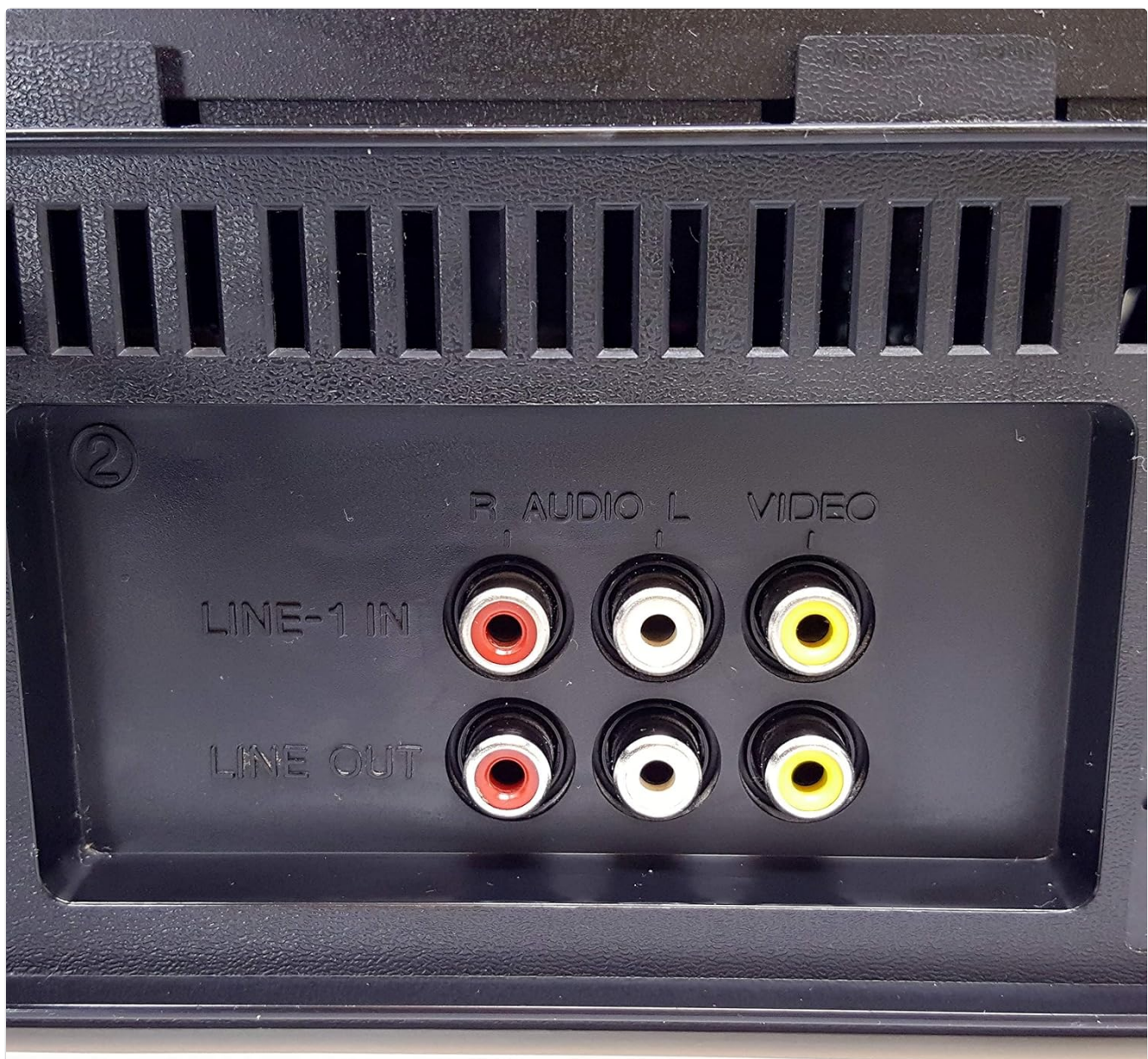
Image: Close-up of the rear audio/video input and output jacks.
